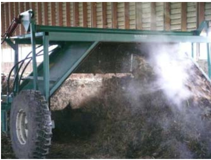
Windrow composting of carcasses using low-carbon composting techniques and Sittler compost turner.
