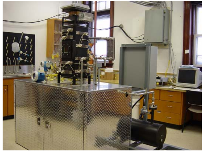
Figure: Superheated steam dryer used to determine the physical and textural properties of noodles.
