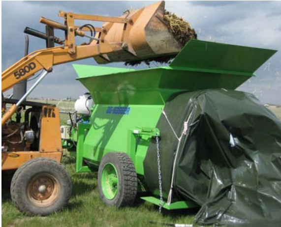
Filling of the composting bag with feedlot manure and monitoring of the temperature inside.
